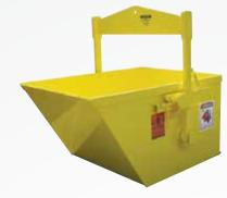
The Hippo Hopper Self-Dumping Crane Hopper is designed for use in manufacturing plants and commercial construction. The hopper can be maneuvered into place with an overhead crane and easily dumped by pulling down on the lever for a full 90 degree dump.
